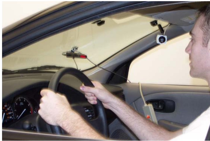
Figure 5. View of SWS receiver mounted on the middle of the windshield
