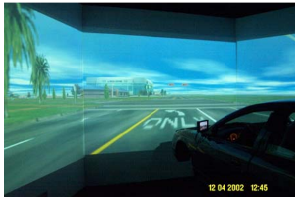
Figure 3. Simulator screens showing wide field of view
