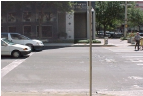
An example of an advance stop line relocated 20 feet in front of the crosswalk.
