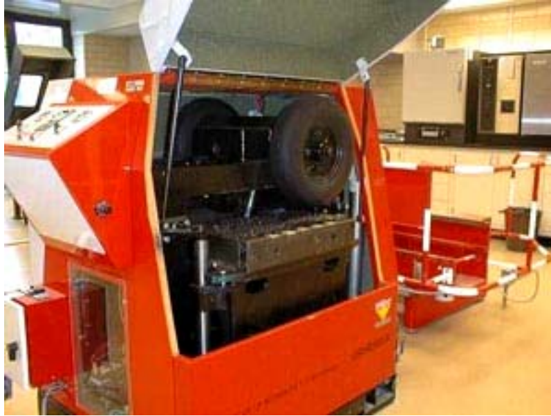
Figure 2-10. The French pavement rutting tester.
