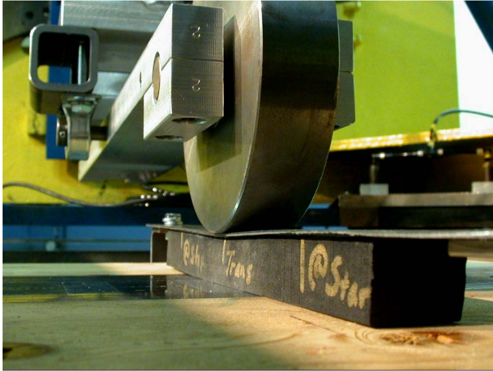
Figure 3-14. Close-up picture of the loading strip test.
