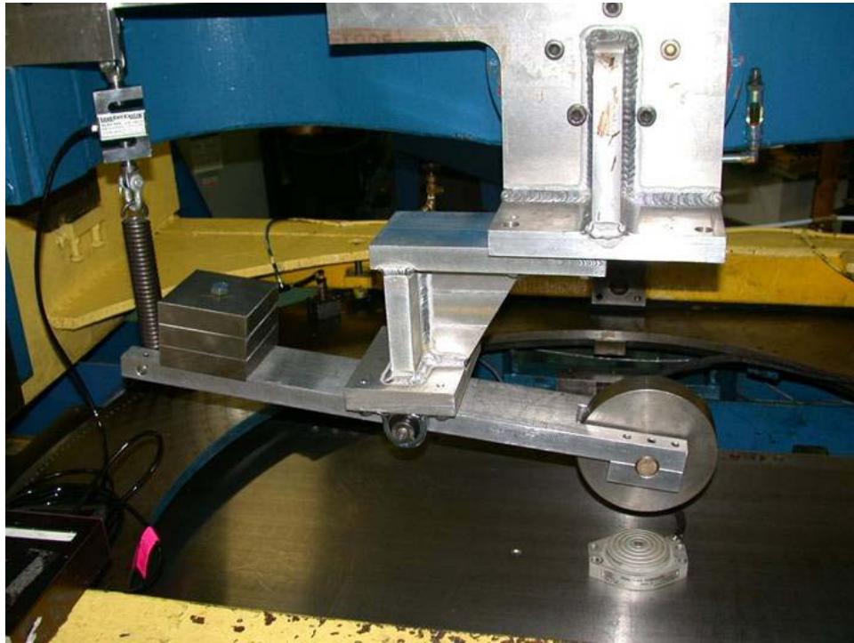
Figure 3-11. Contact stress measuring apparatus setup and calibration.
