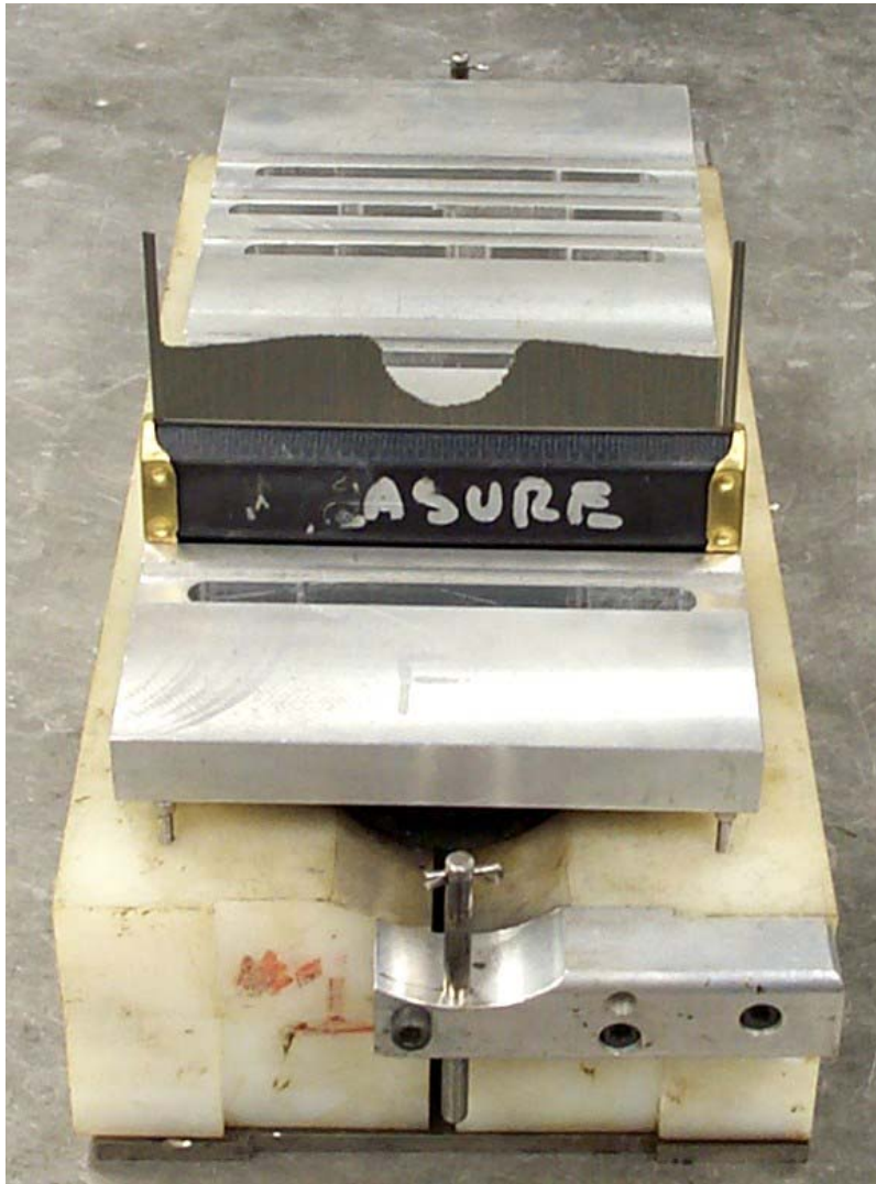
Figure 5-7. Contour gauge measuring the surface profile of the specimen.
