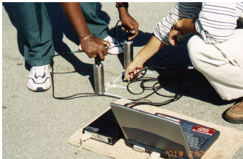
Figure 5-5. Crack Depth Measurement Using Impact Echo Testing System
