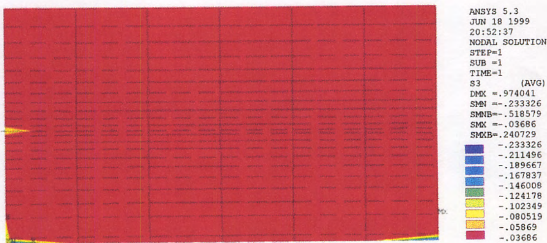
Fig. 5.10 Principal stress distribution from finite element analysis for HDPE geogrid in sand under unsaturated condition (10% Pult)
