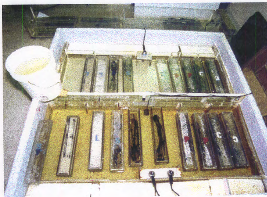
Figure 8.3 Uncovered durability tanks
