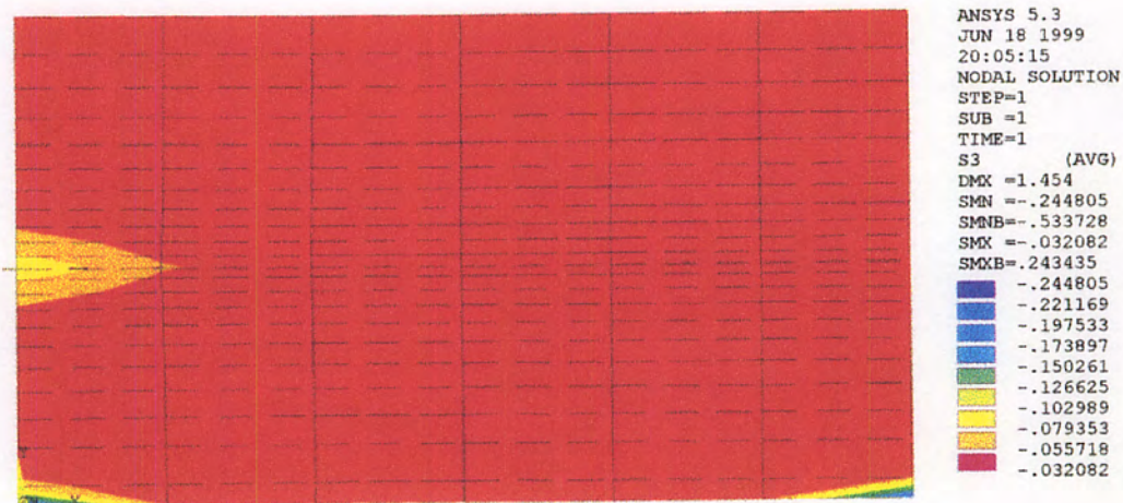
Fig. 5.11 Principal stress distribution from finite element analysis for HDPE geogrid in sand under unsaturated condition (25% Pult)
