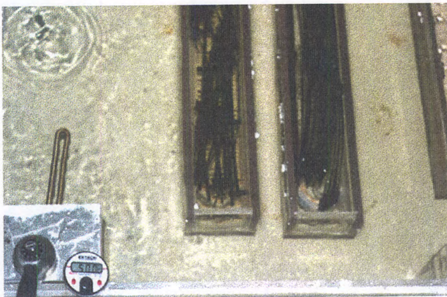
Figure 8.6 Temperature control, 50° C tank
