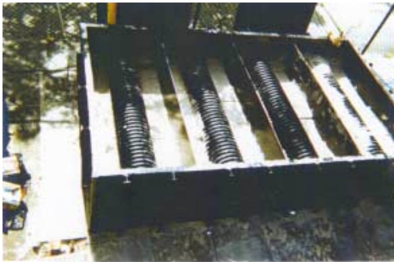
Fig. 3.21 Soil chambers (half full) after compaction
