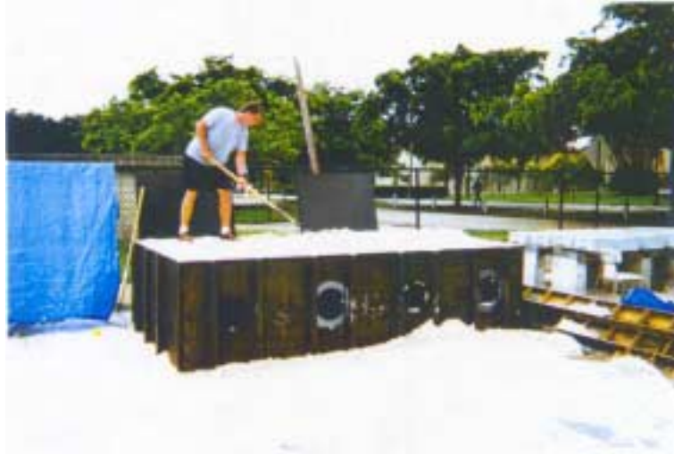
Fig. 3.22 Soil chambers (full) after compaction
