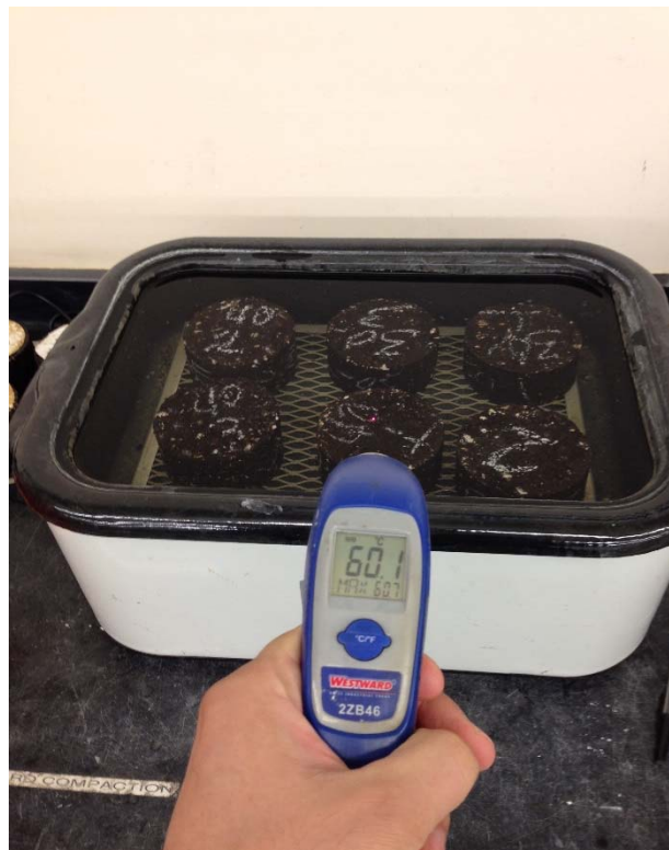
Figure 6.8: Wet subsets, soaking in distilled water at 60 °C for 24 hours
