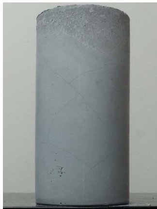
(f) B20 Minor longitudinal and transverse cracks
