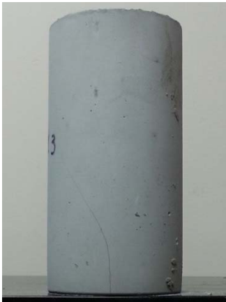
(b) F10 Minor longitudinal cracks
