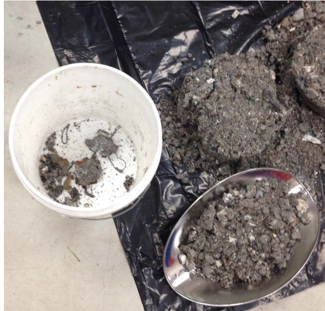
Figure 6.1: Visual inspection of BA aggregate
