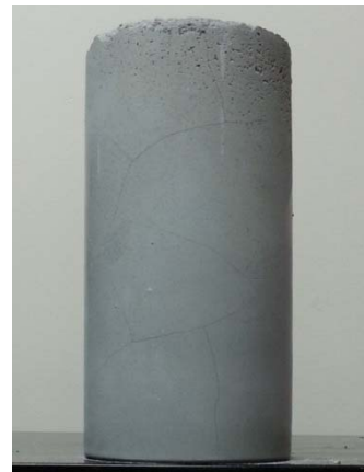
(g) B30 Moderate longitudinal and transverse cracks
