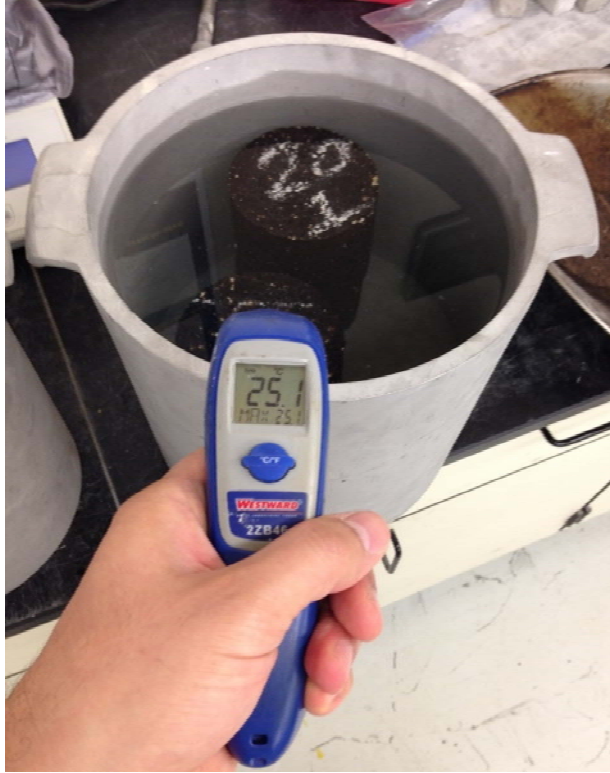
Figure 6.9: Wet subsets, adjusting the temperature by soaking in a water bath at 25 °C
