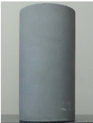
(e) B10 Minor longitudinal cracks
