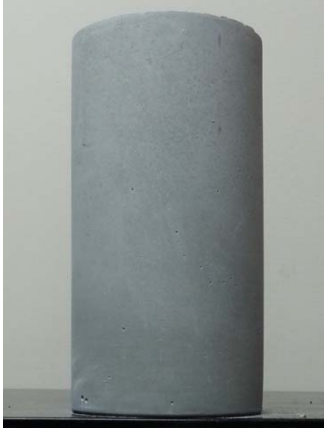
(a) C No cracks or voids
