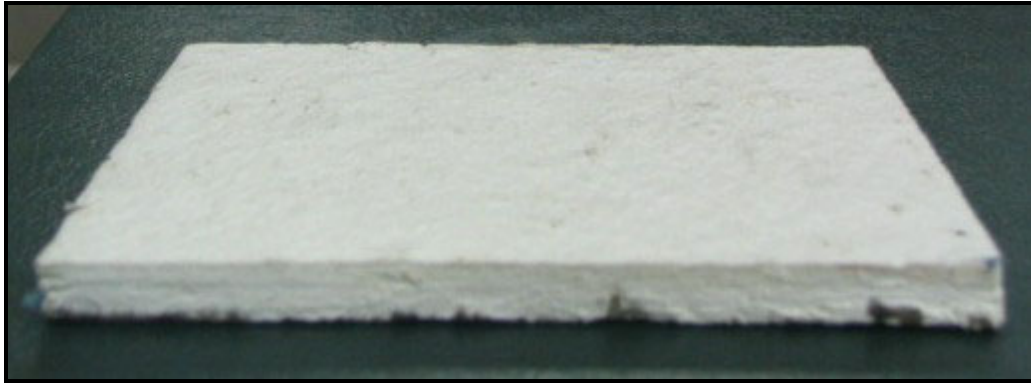
Photograph 2. Sectional view of temporary rumble strip
