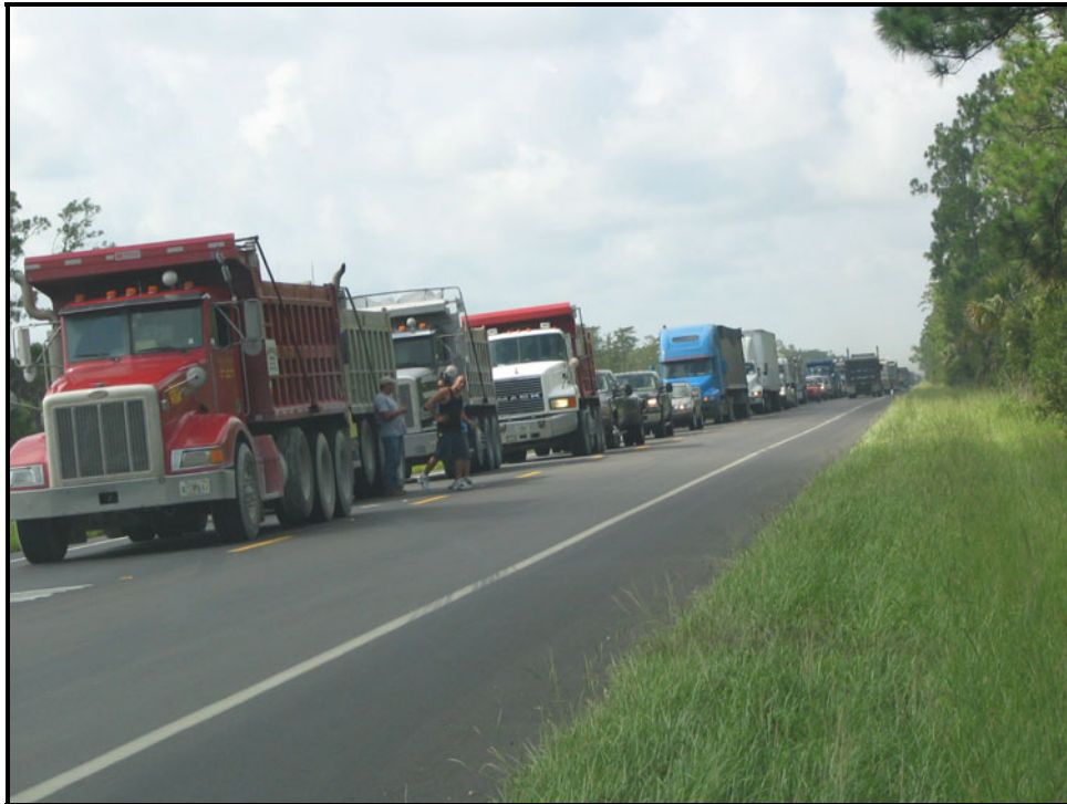
Photograph 6. Typical Queue Buildup due to One-Lane Operation
