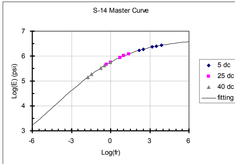
Figure 7-28. Master Curve for S-14 mixture
