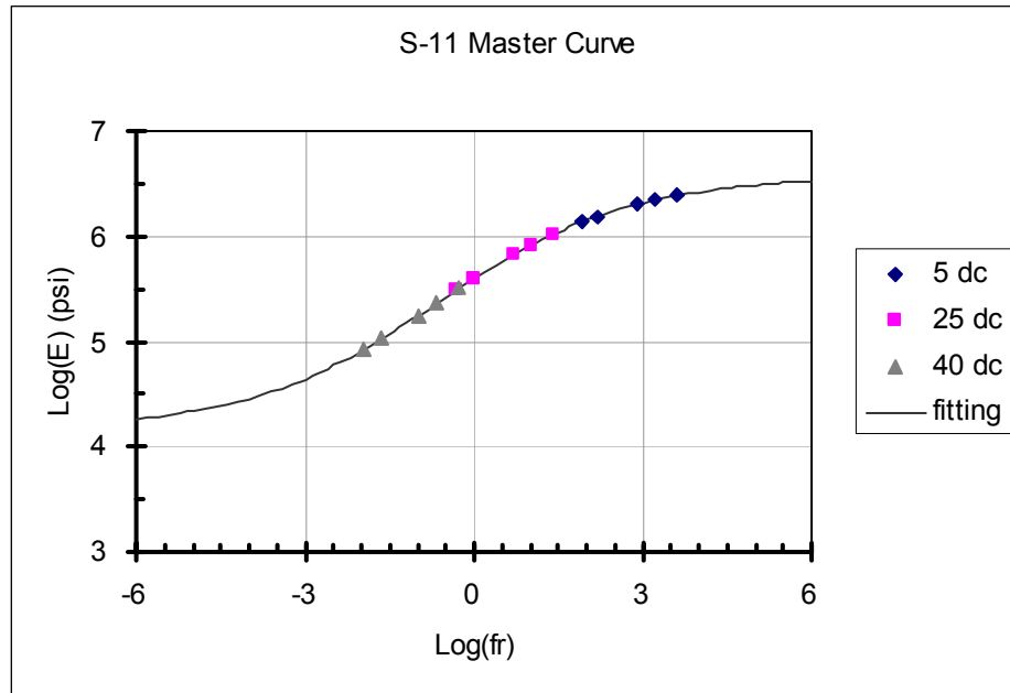
Figure 7-22. Master Curve for S-11 mixture
