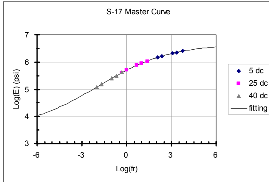
Figure 7-34. Master Curve for S-17 mixture
