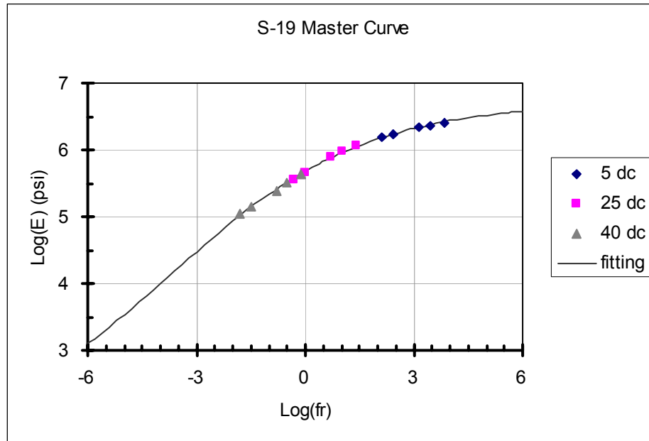
Figure 7-38. Master Curve for S-19 mixture
