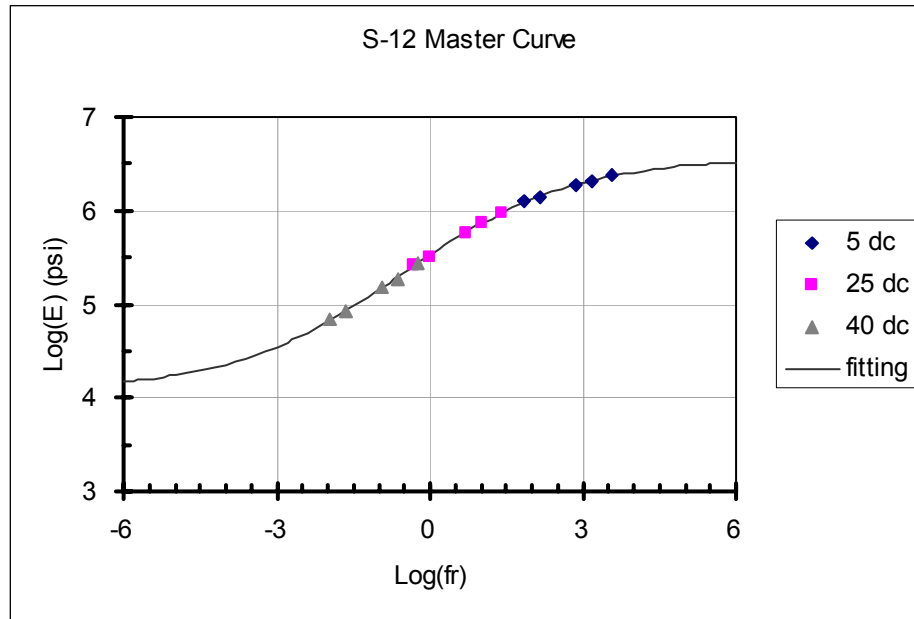
Figure 7-24. Master Curve for S-12 mixture
