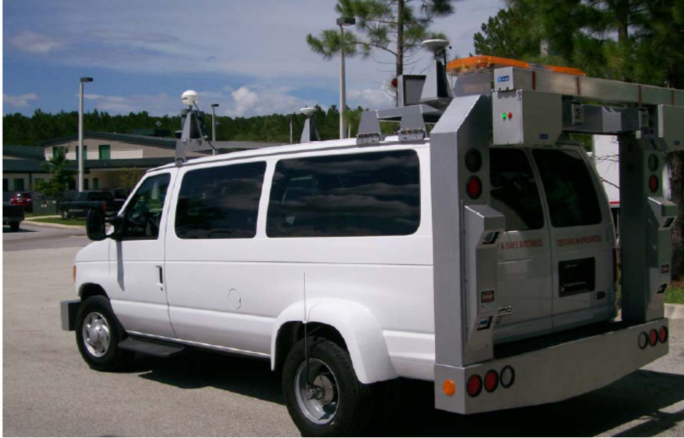
FIGURE 2 FDOT High Speed Inertial Profiler (HSIP)
