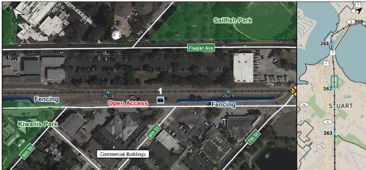
In Downtown Stuart, a gap exists in the existing fencing allowing for open access to the railroad tracks (photo 1). Further north of the city, Stuart has provided a 4 ft. aluminum fence on both sides of the corridor that ends just to the south end of Kiwanis Park at 5<sup>th</sup> St. From 6<sup>th</sup> St. to 7<sup>th</sup> St., a 4 ft. chain link fence was installed, leaving a gap between 5<sup>th</sup> St. and 6<sup>th</sup> St.
