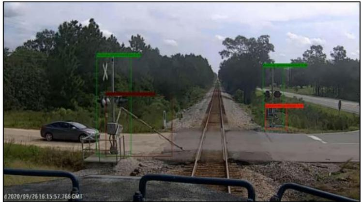
Figure 9: Video Detection Algorithm - Wi-Tronix using Locomotive Camera
