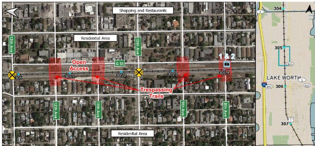
Between 13<sup>th</sup> Ave. and 7<sup>th</sup> Ave. (not shown, MP 305.5) in Lake Worth, the right-of-way has open access with little to no vegetation or barriers between the parallel G St. (photo 1). Well-established paths cross the tracks to G St. from the dead-end streets on the west side of the corridor (photo 2).
