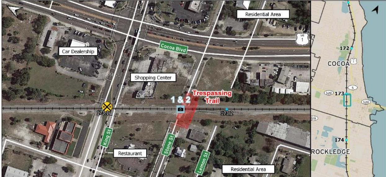
In Cocoa, a well-defined footpath crosses the tracks at the dead end street, Stone St. In 2007, the grade crossing was closed, and the crossing panels and sidewalks were removed. However, a trespassing trail developed in its place between the remaining sidewalks on either side of the crossing (photos 1 and 2).
