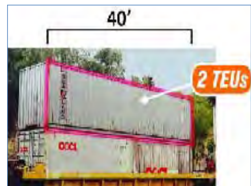
A two TEU is 40 feet long and is equivalent to two single containers.
