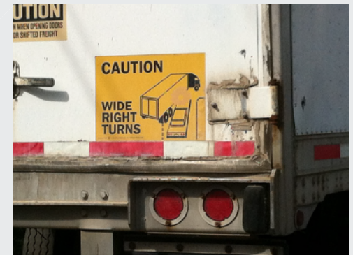
Turning movements by large vehicles are complicated by both a wide turning radius and blind spots.
