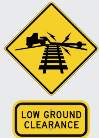
The low ground clearance warning can be used to notify trucks departing a state highway of a nearby local road constraint.
