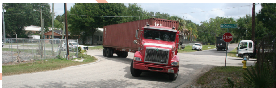
Although there is only a slight difference in width between trucks and other passenger vehicles, trucks have other operating characteristics due to greater height, length, and center of gravity that affect visibility and maneuverability.
