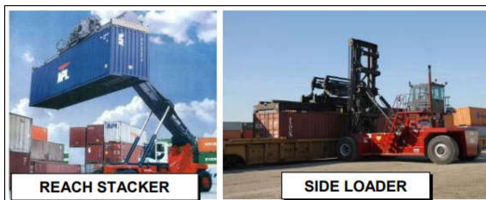
Figure 4-13: Reach Stacker and Side Loader Cranes
