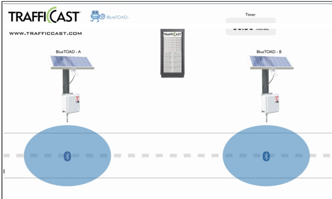
Figure 2. How Bluetooth Technology Works with BlueTOAD
