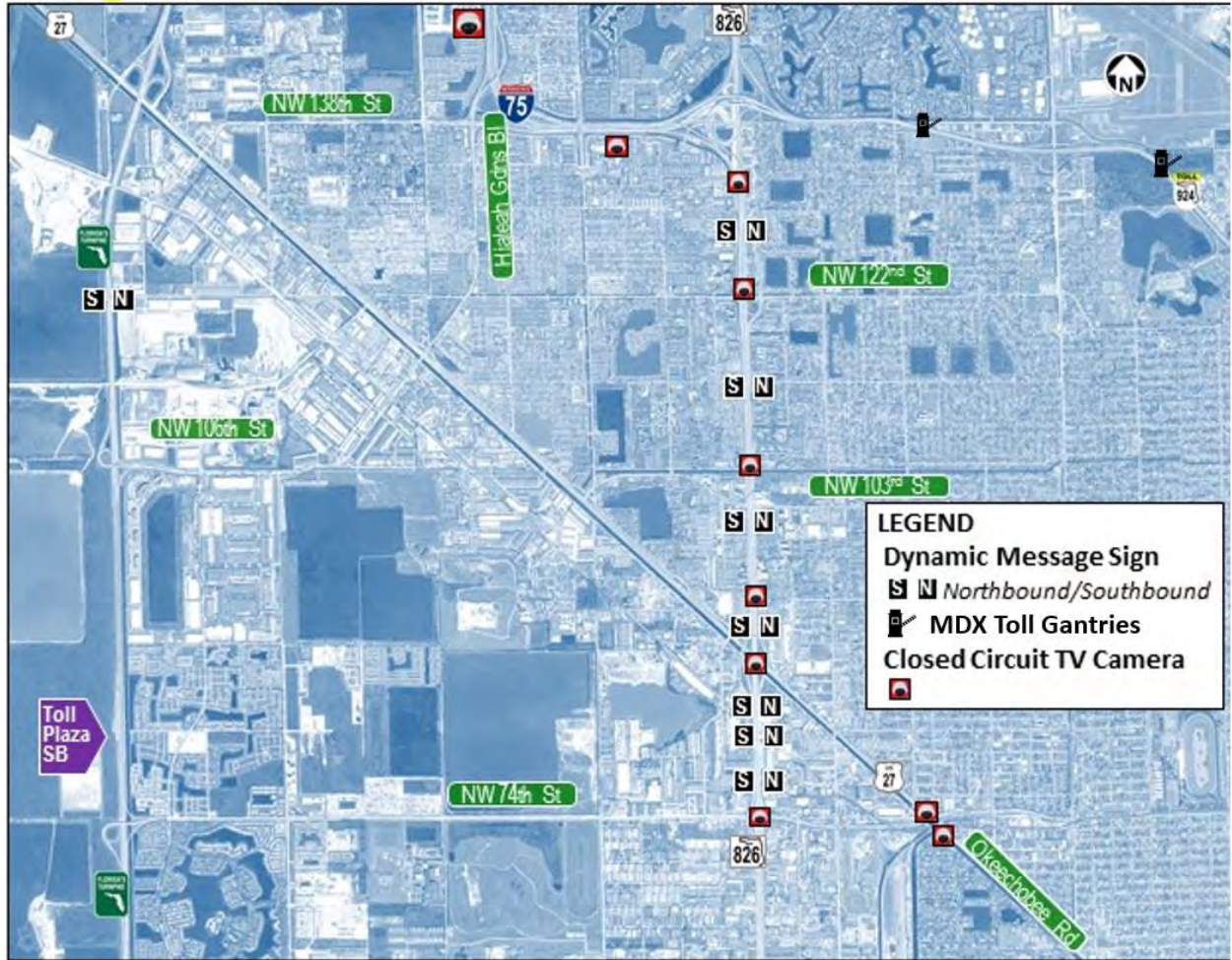
Figure 1-17: Existing ITS Infrastructure in the Vicinity of the Town of Medley
