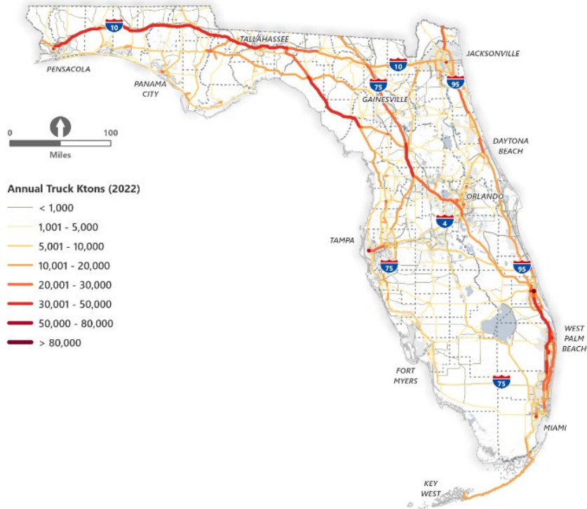
Figure 6 | Freight Analysis Framework Roadway Tonnage (Ktons) Moved in Florida, 2022 and 2050
