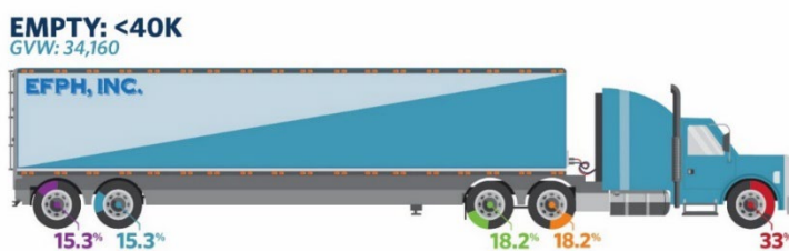
Figure 4 | Class 9 Truck Axle Weight Load Distribution
