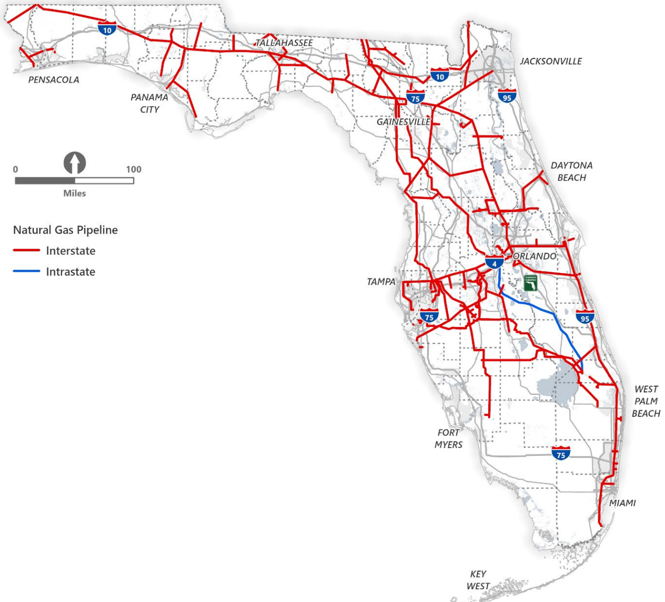
Figure 5 | Florida’s Natural Gas Interstate and Intrastate Pipelines
