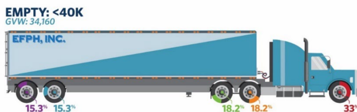
Figure 4 | Class 9 Truck Axle Weight Load Distribution
