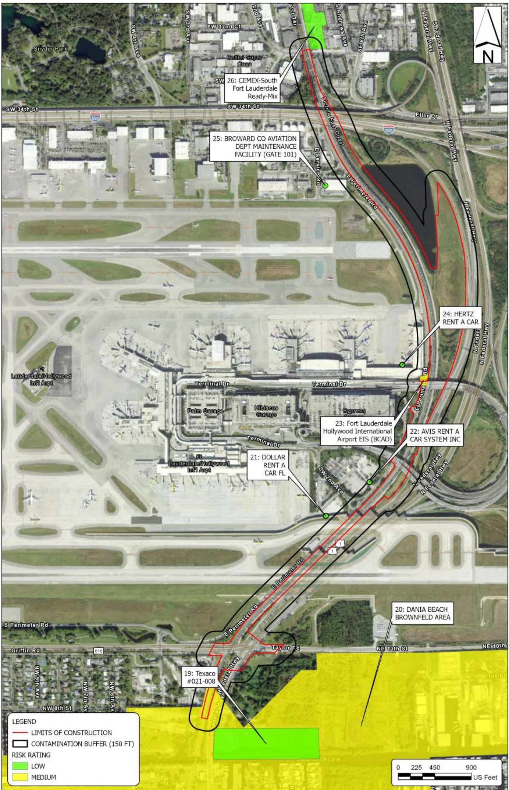
Figure 3-10: Potential Contamination Risk at FLL Airport Station
