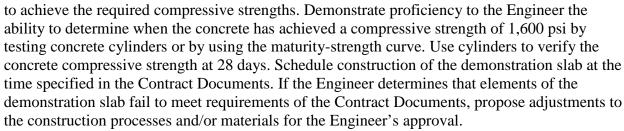
The demonstration slab may be used in the final work with the approval of the Engineer. No slab replacements will be constructed until the demonstration slab is approved. The Engineer may require additional demonstration slabs until a demonstration slab conforms to the Contract Documents.
