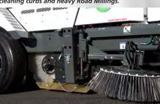
DUST SUPPRESSION SYSTEM • Global M4HSD includes 280 Gallon Water Tank Capacity combined with Two(2) Diaphragm Water pumps and Two(2) Modes (LOW/ HIGH) provide versatility and superb dust control.
