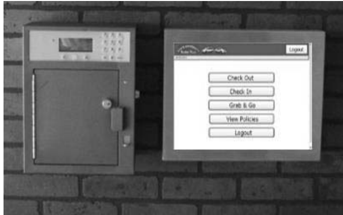
A standard self-service motor pool consists of a key control device (on left) and a full-color, touch-screen kiosk (on right)
