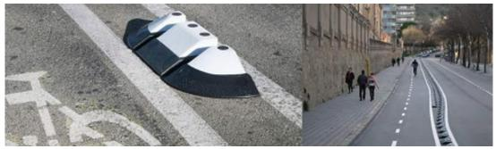
Figure 12: Photos of Zipper Delineators in Use
