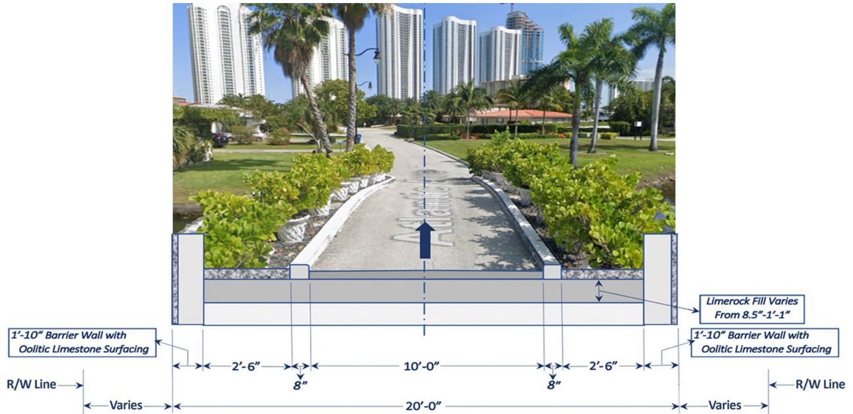
Figure 2-10. Existing Atlantic Avenue Bridge (No. 874218) Typical Section
