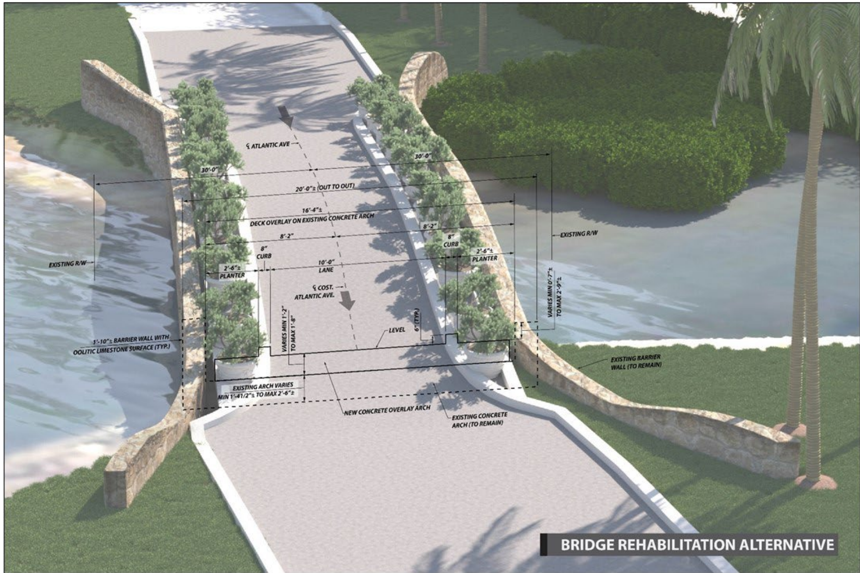
Figure 4-1. Build Alternative 1 – Rehabilitation, Proposed Typical Section
