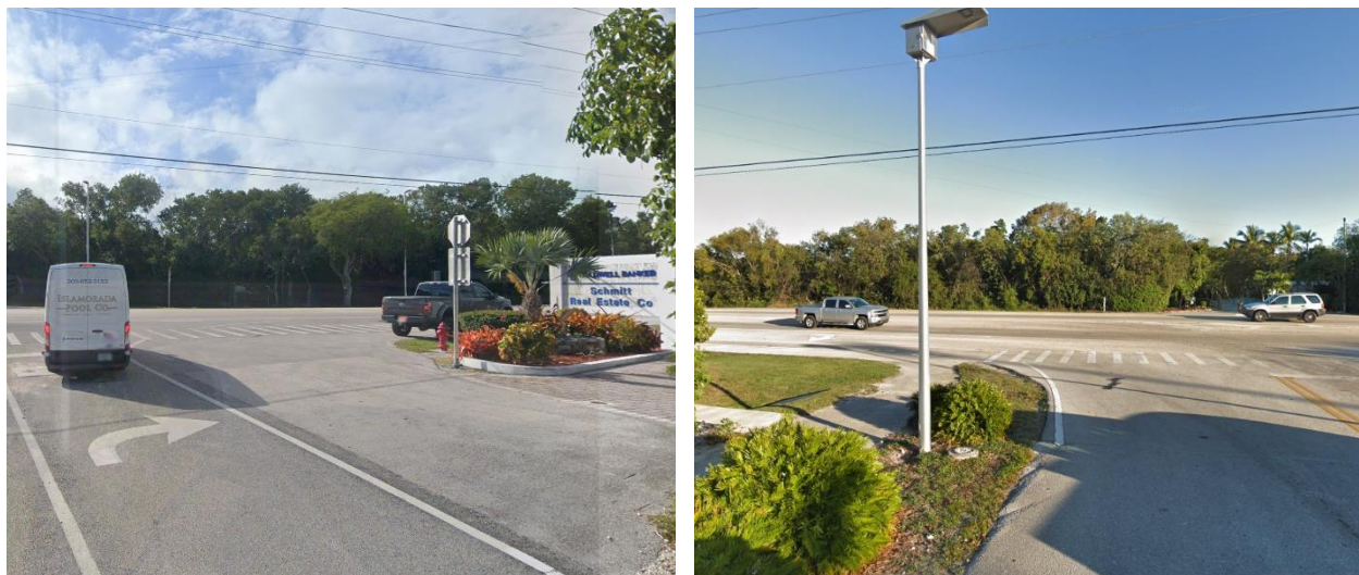
Figure 2-6 Clear Sight obstructions at intersections
