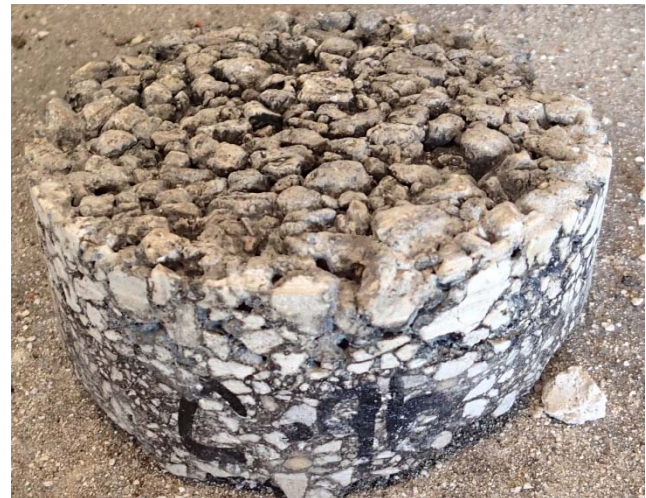
Partial Core Unable to fully extract core from bridge deck.
