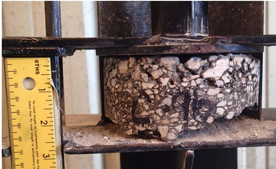
Partial Core Unable to fully extract core from bridge deck.
