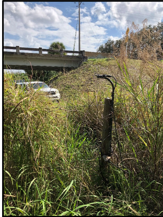
Photo 3 – U1 ultrasonic microphone placement above the shrub zone using bracketed mount on a fence pole at survey Site 2. Microphone is approximately 5 feet above ground (to minimize potential for equipment theft/vandalism) and facing open areas to reduce interference from vegetation and maximize potential number of recordings.
