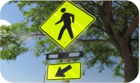
Rectangular Rapid Flashing Beacon
