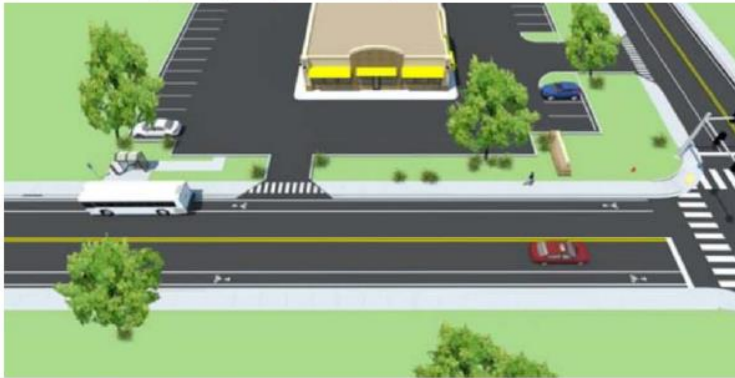
Figure 103 | Acceptable Bus Stop Placement Near Driveway
