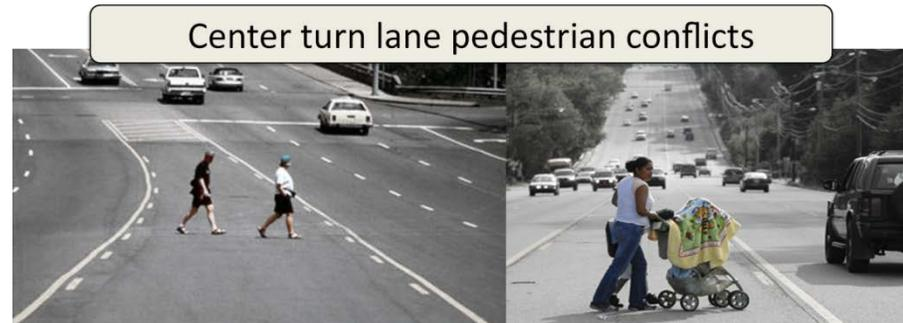
The task of a pedestrian crossing the street is more challenging without a restrictive median. Pedestrians need to be aware of drivers in both directions and are not as visible to a driver traveling at a higher speed.
