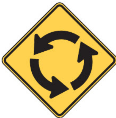
Figure 5-7 Advance Warning Signs for Roundabouts (W2-6)
