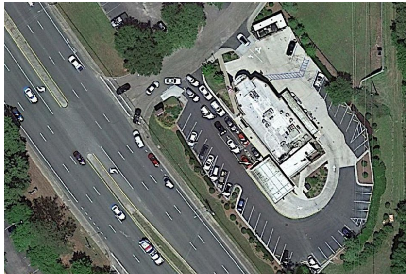
Figure 27 | Inadequate Site Design with Drive-Through Queue Backup onto Arterial
