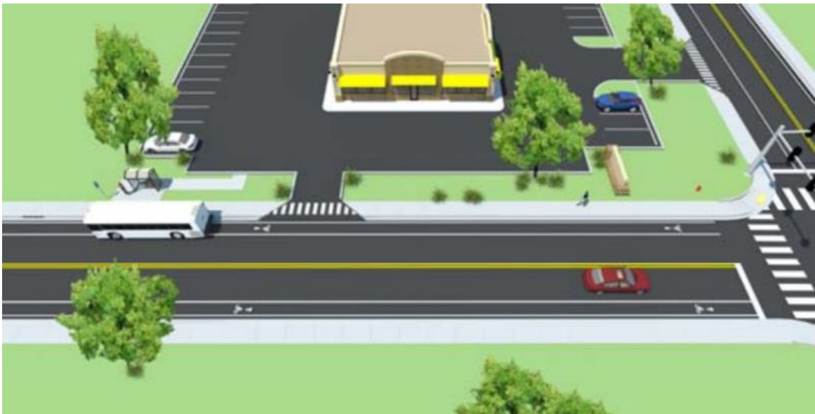
Figure 103 | Acceptable Bus Stop Placement Near Driveway
