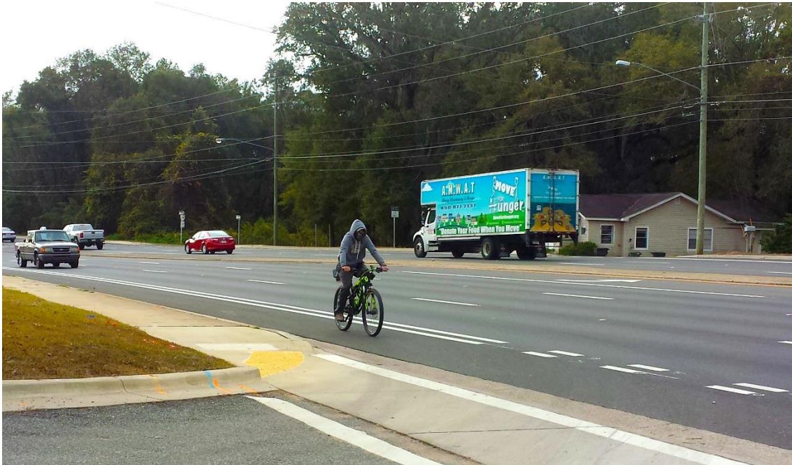
Figure 86 – Buffered Bike Lanes in Freight/Industrial Areas
