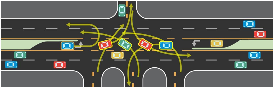
Figure 32 – Vehicles Stopped in Excessively Wide Median Opening
