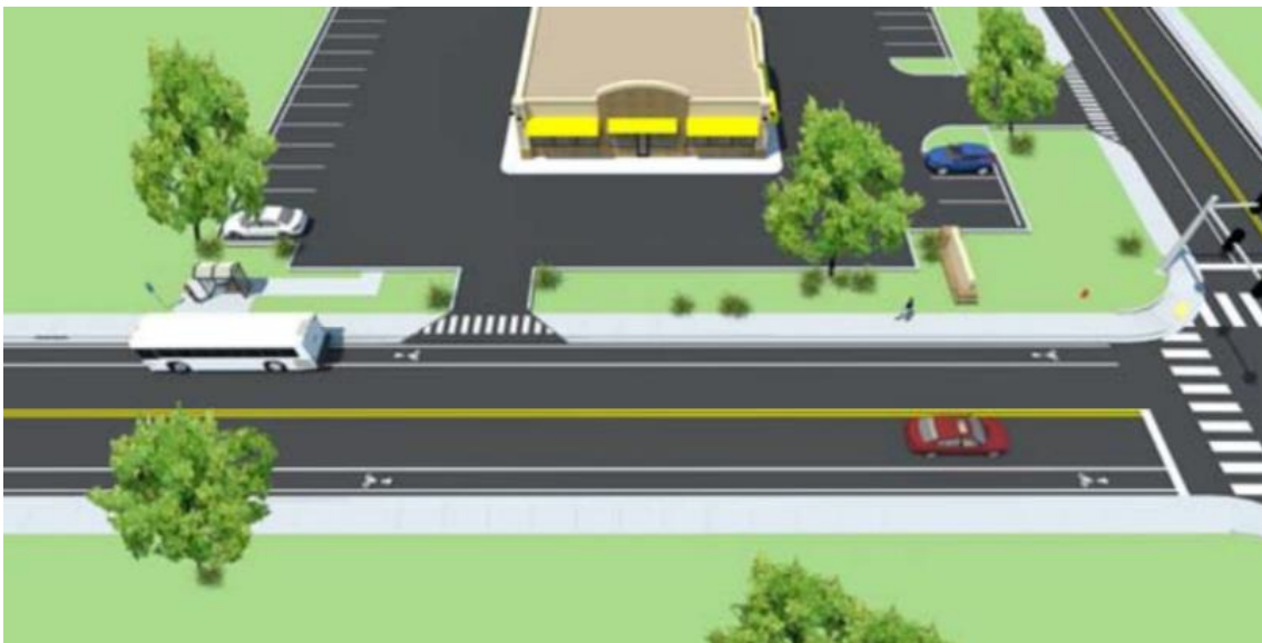
Figure 89 – Acceptable Bus Stop Placement Near Driveway
