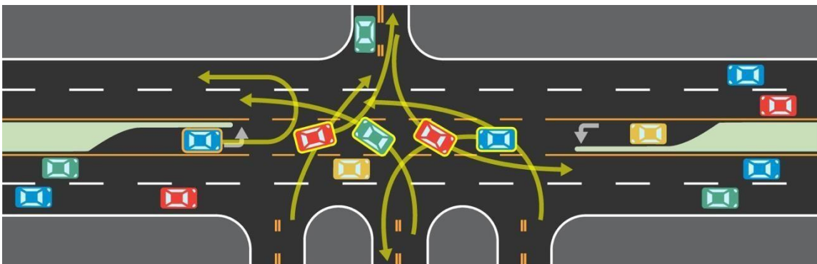
Figure 41 | Vehicles Stopped in Excessively Wide Median Opening
