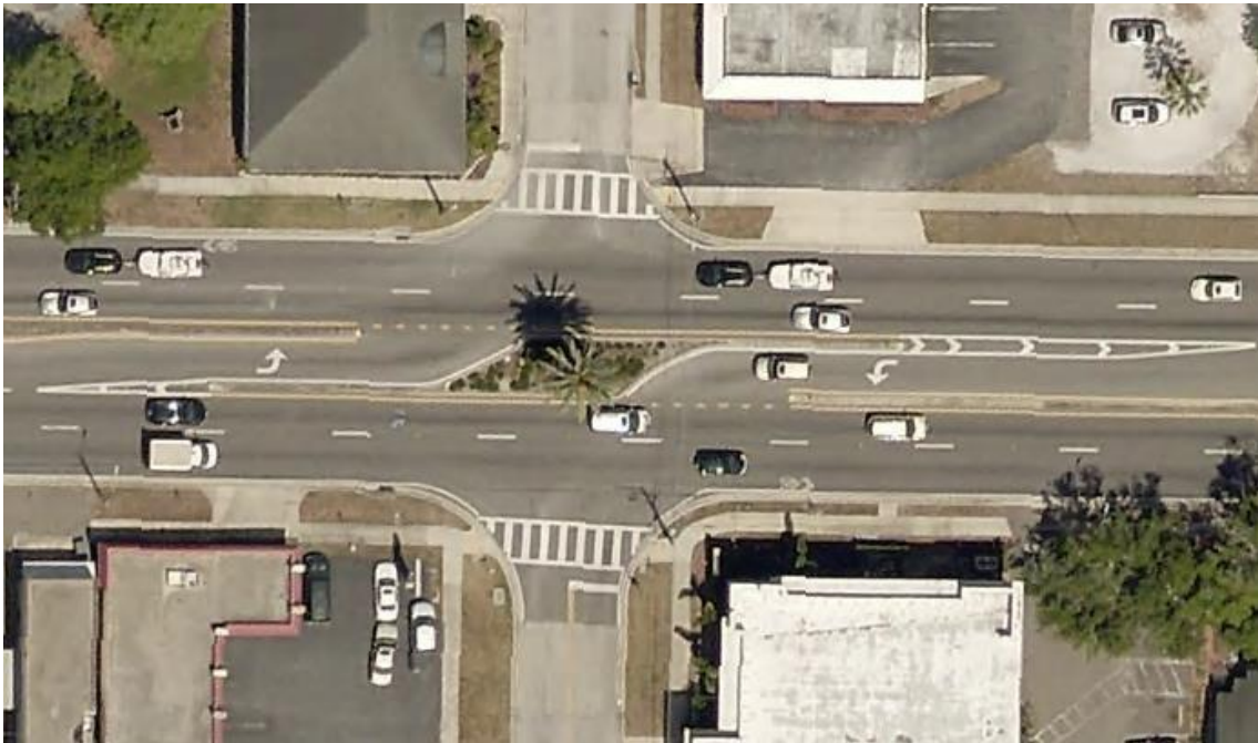
Figure 14 | Example of a Dual Directional Median Opening
