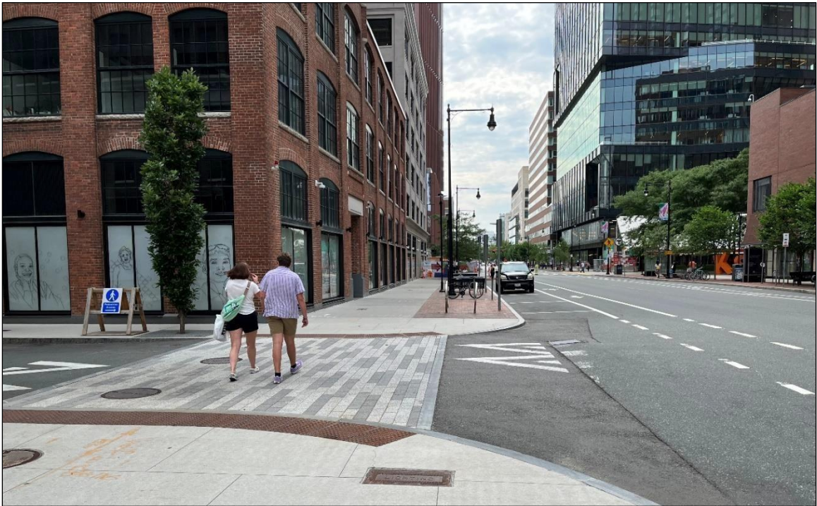
Figure 60 | Raised Sidewalk Crossing
