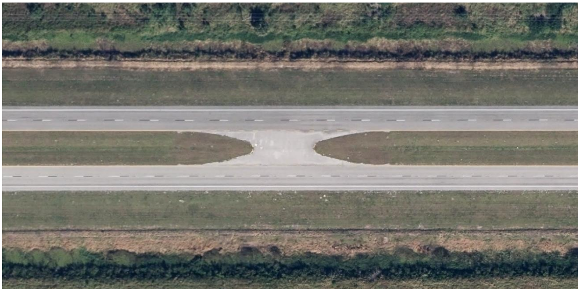
Figure 13 | Example of a Full Median Opening
