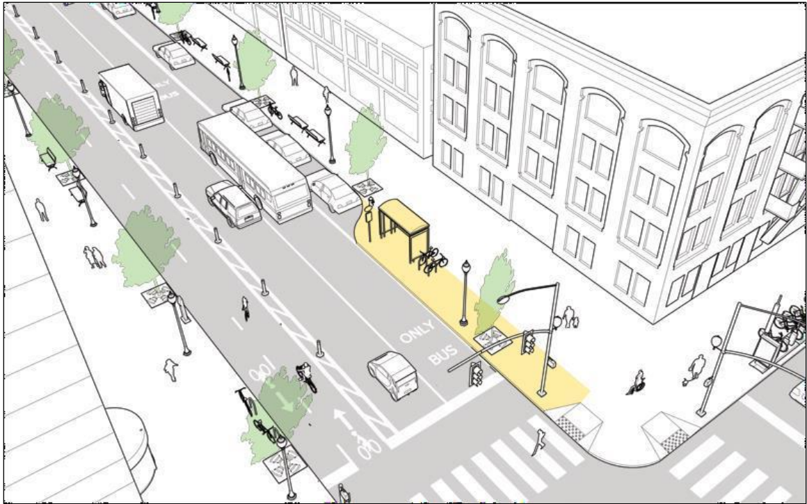
Figure 147 | Graphic of a Bus Bulb
