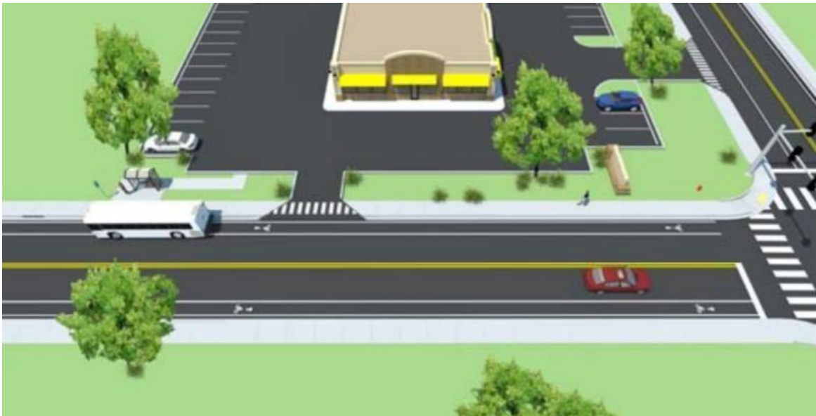
Figure 103 | Acceptable Bus Stop Placement Near Driveway
