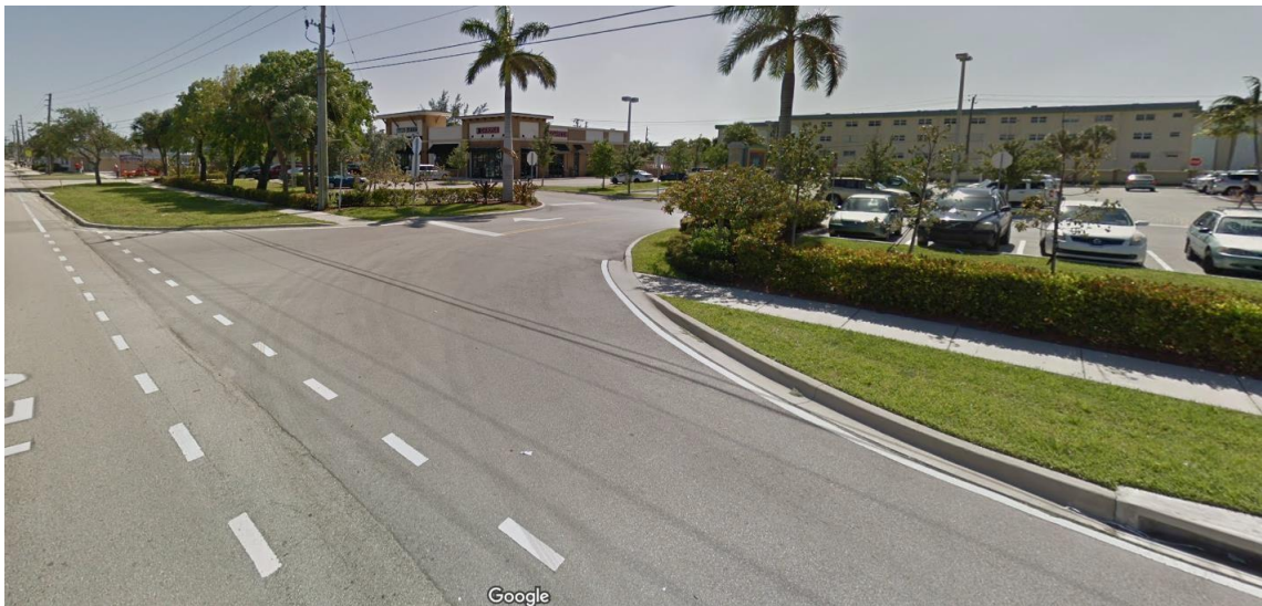
Figure 10 | Curbed Roadway (Radial Return)
