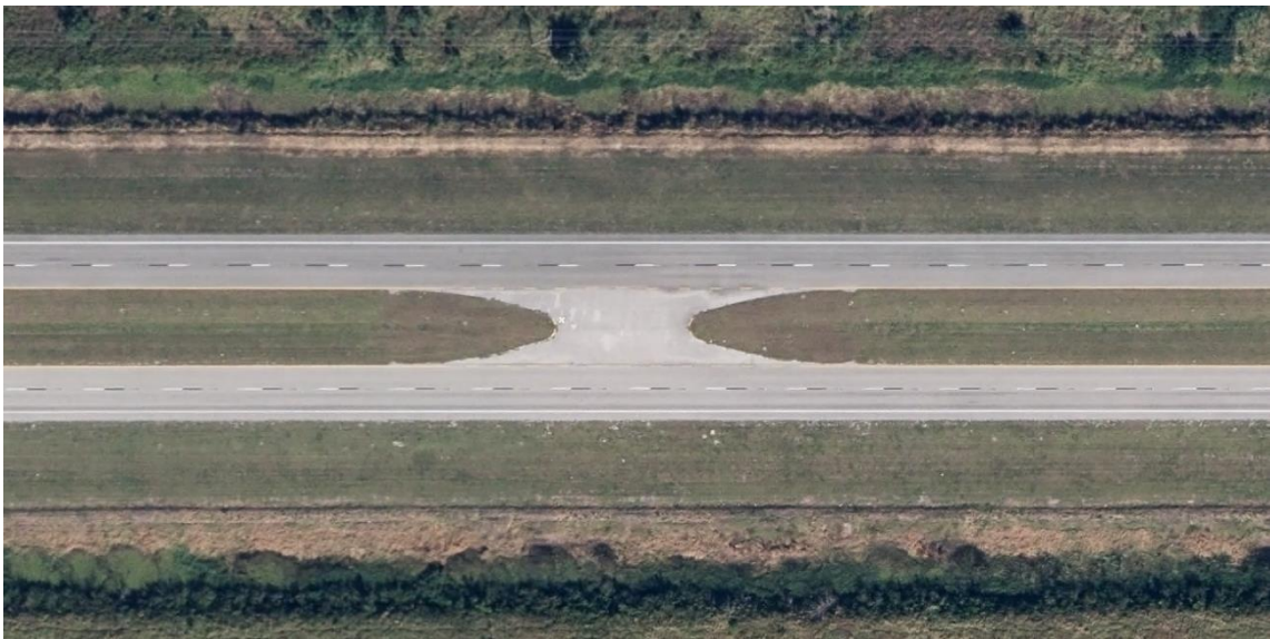
Figure 13 | Example of a Full Median Opening
