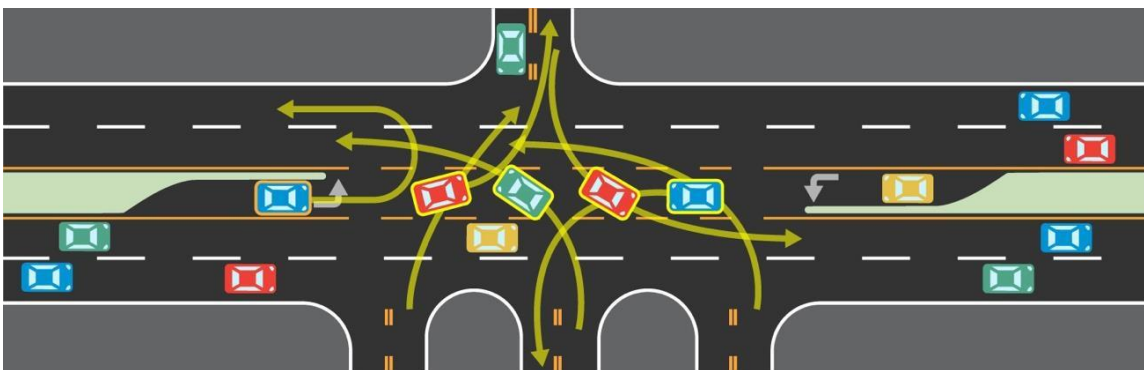
Figure 41 | Vehicles Stopped in Excessively Wide Median Opening
