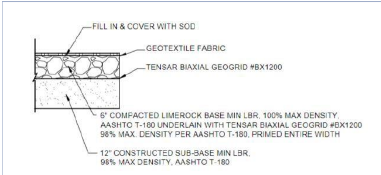
Figure 24 | Example Emergency Access Driveway Stabilization Detail
