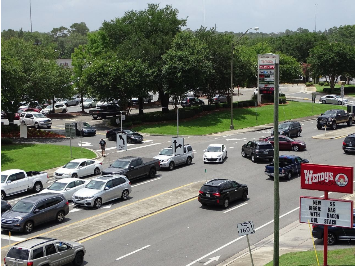
Figure 40 | Vehicles Stopped in Excessively Wide Median Opening
