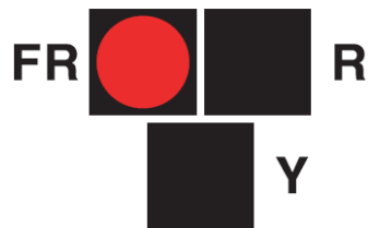
5. Alternating Flashing Red During Pedestrian Clearance Interval
