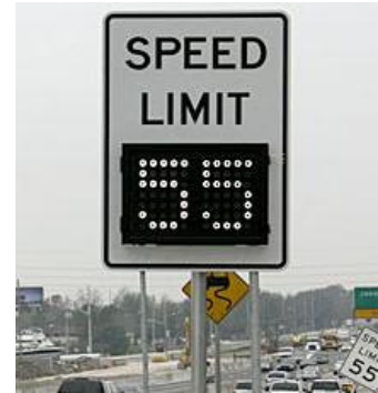
Figure 3-3: Example Variable Speed Limit Sign
