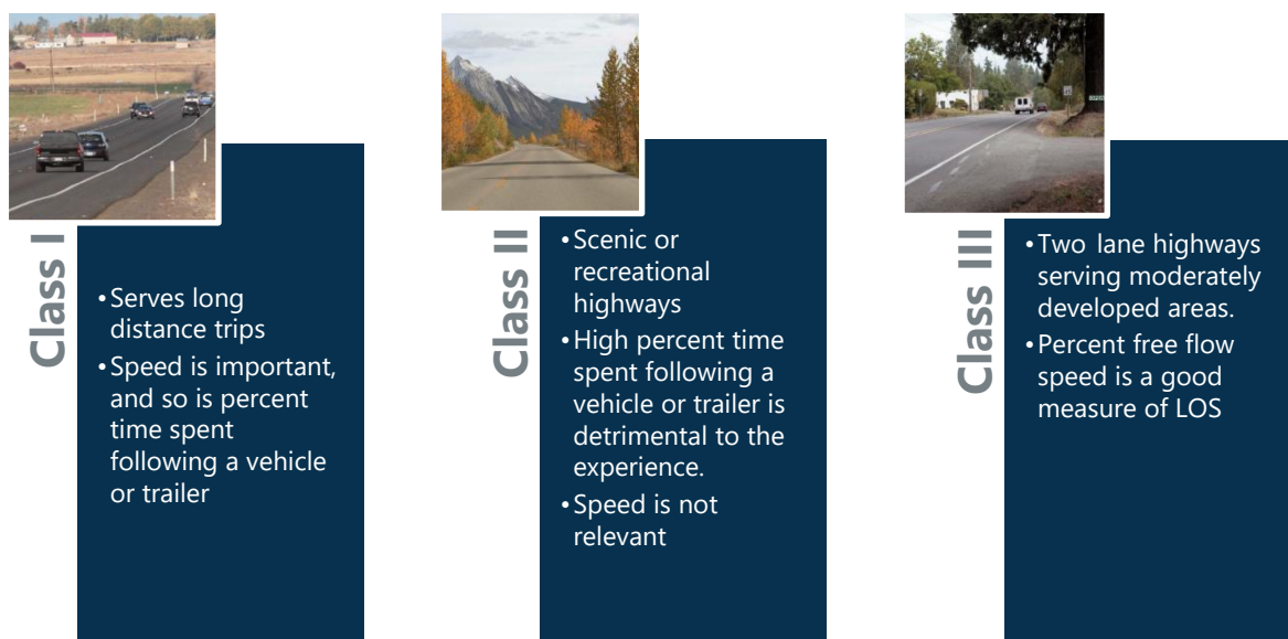
Figure G.1 Two-Lane Highway Classification
