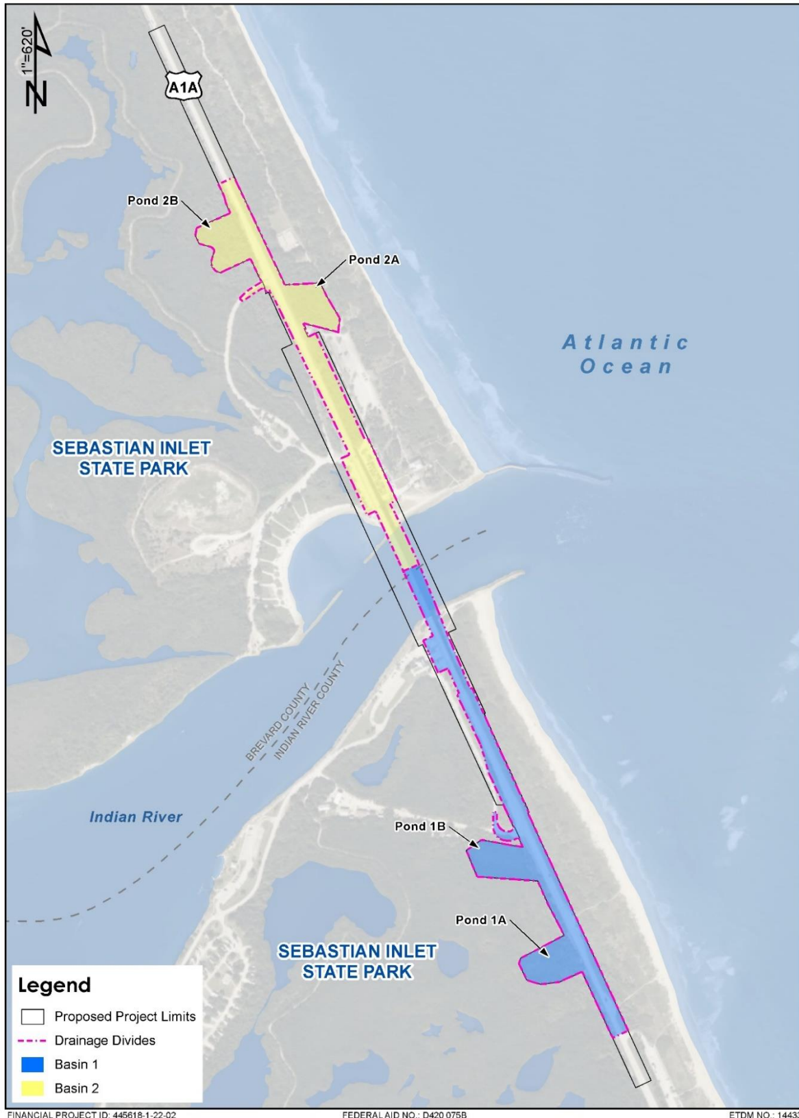
FIGURE 6-4: STORMWATER POND ALTERNATIVES
