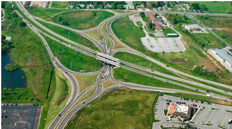
– B – Overpass DDI Source: Tennessee DOT
