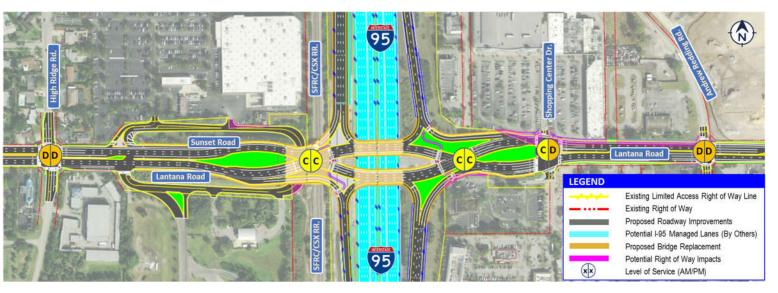
**Build Alternative 2** with the Diverging Diamond Interchange (DDI) configuration was selected as the preferred alternative due to the following advantages it possesses over the other two build alternatives:
