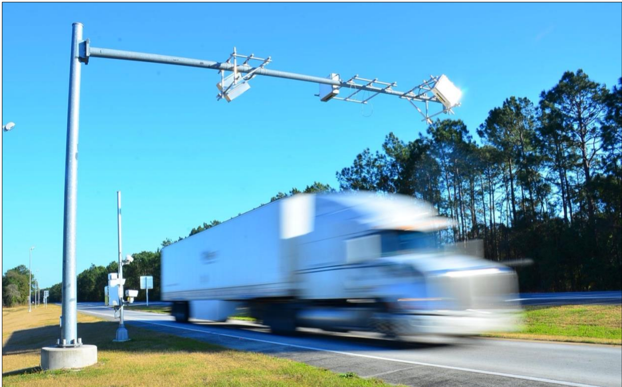
Figure 2. Commercial vehicle passing over Weigh in Motion (WIM) and size detection screening.
