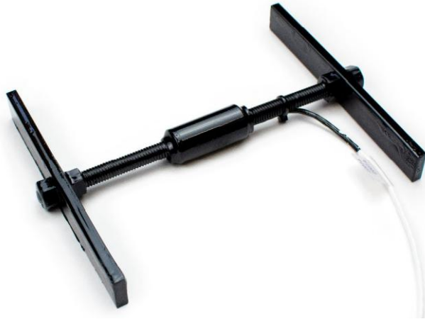
Figure 6 Asphalt Strain Gauge
