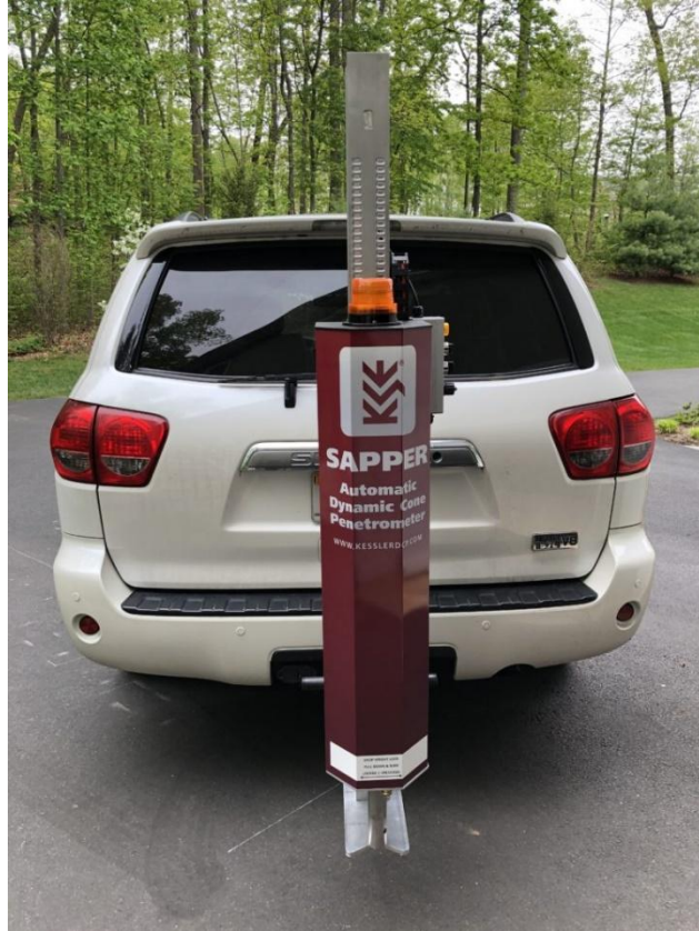
Figure 13. DCP Device, SAPPER Automatic Dynamic Cone Penetrometer
