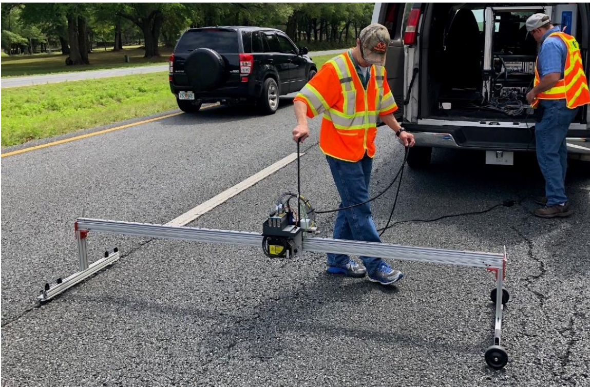
Figure 3. Florida Laser Meter (FLM) used for rut and fault depth verification.
