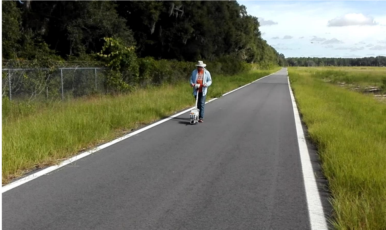
Figure 2. SurPro Collecting Reference Longitudinal Profile for AASHTO R56 Certification.
