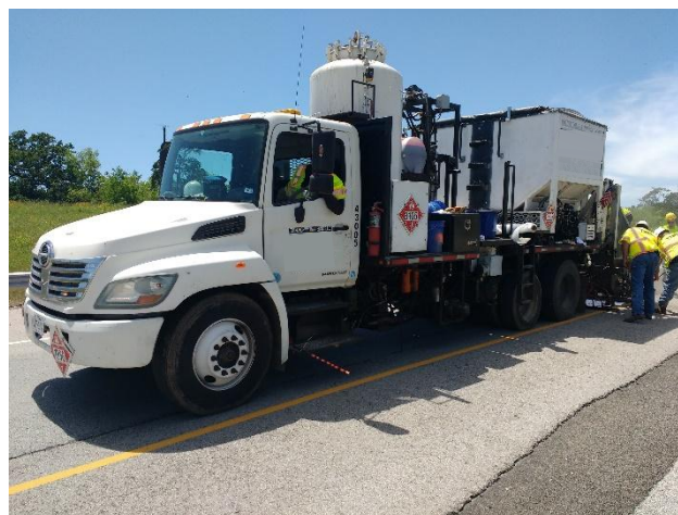
FIGURE 10 – Continuous automated HFST applicator vehicles. (9)
