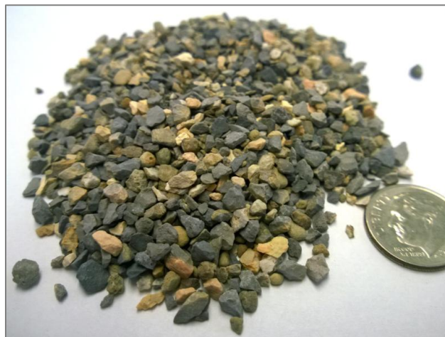
FIGURE 7 – Calcined bauxite, crushed and graded.
