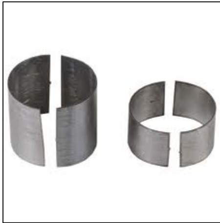
Figure 5. Picture of Shims that Can Be Used to Accommodate a Core Sample with a Diameter Less than 6.0 in.
